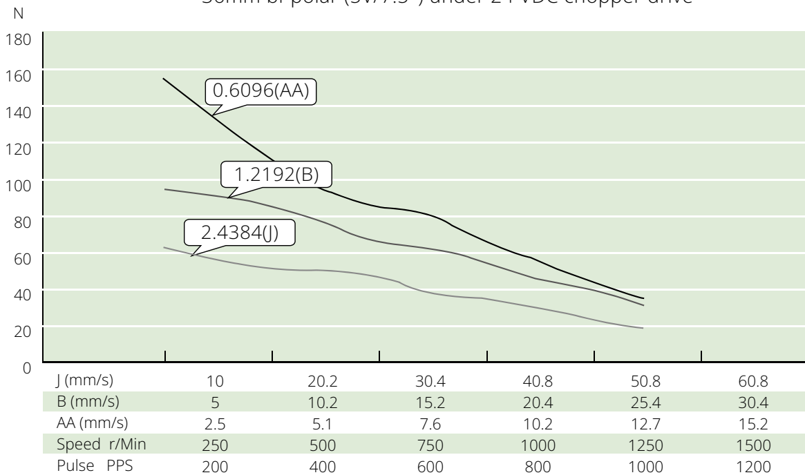
36mm bi-polar (5V/7.5°) under 24 VDC chopper drive
