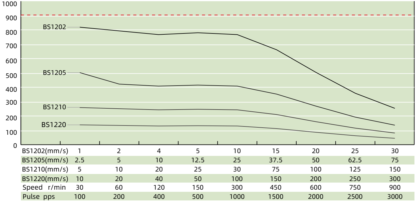
Size 23 Double Stack Speed Thrust Curves
