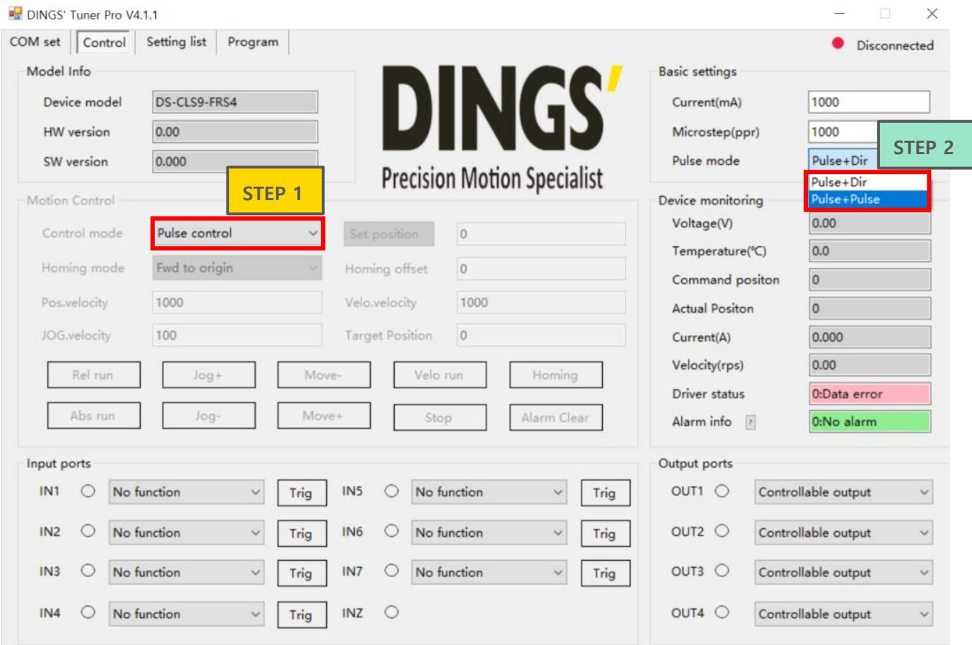
\*In the [ Control ] tab, automatically saves parameters, if you make changes.
