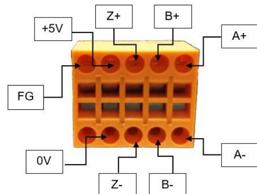
**Pay attention to the polarity of the encoder power supply when wiring**
